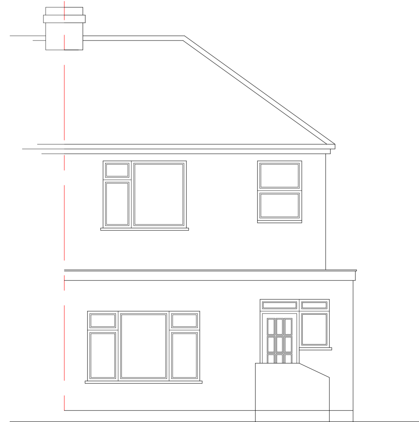
EXISTING REAR ELEVATION 1:50
