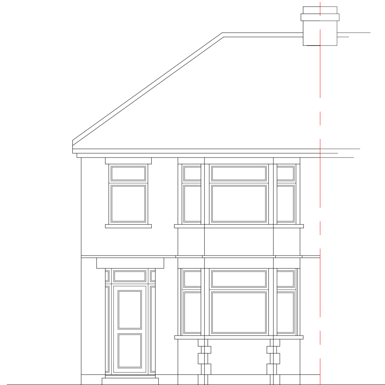
EXISTING FRONT ELEVATION 1:50
